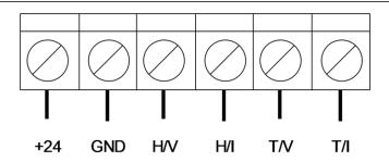
+24: +24Vdc power supply GND: power supply ground
