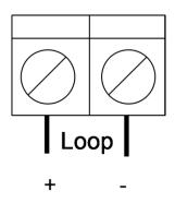
Avoid applying voltages greater than 30VDC.
