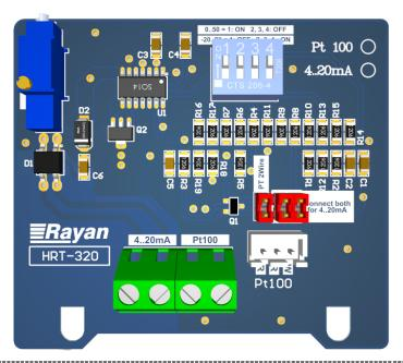
A four-row DIP switch is located on the electronic circuit of the sensor to specify type of output signal range in case of 4...20mA usage.
